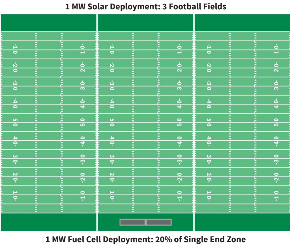
A comparison of the surface area needed for 1 MW of installed solar capacity and 1 MW of solid oxide fuel cell capacity. Source: Robert Bosch
