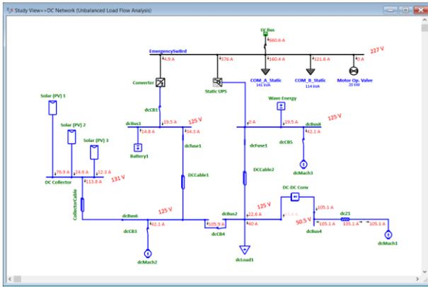
Fig. 9 – Unified AC & DC load flow for a DC Microgrid
