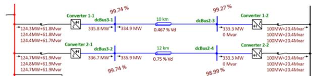
Fig. 8 – AC & DC unified load flow interconnected system
