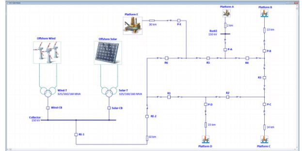
Fig. 2 - Single-line diagram of offshore system
