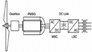
Fig. 4 – WECS PMSG technology
