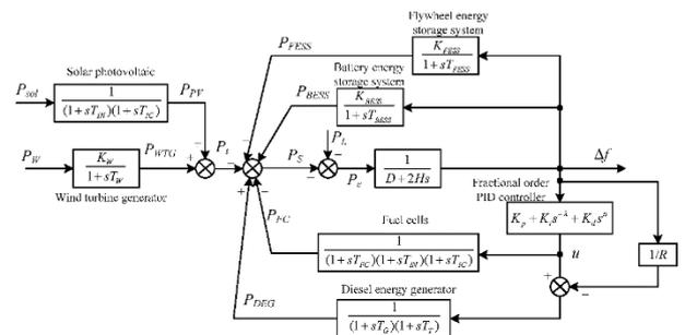
Fig. 15 – Sample frequency control logic
