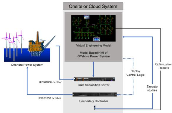
Fig. 16 – Microgrid controller setup for unmanned operation
