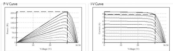
Fig. 5 – Photovoltaic modeling using P-V and I-V curve
