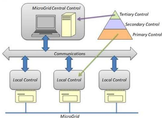
Fig. 13 – Microgrid controller hierarchical controls
