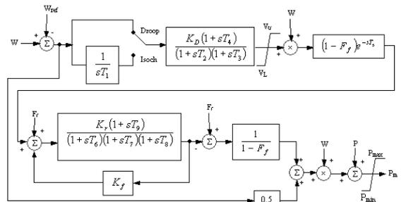
Fig. 3 – Governor model for gas turbine
