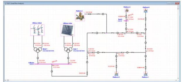
Fig. 12 – Steady-state load flow at rated condition
