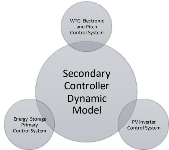
Fig. 14 – Microgrid controller interaction with primary control systems
