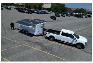
Figure 2: Sesame Solar Nanogrid Easy Set-up
