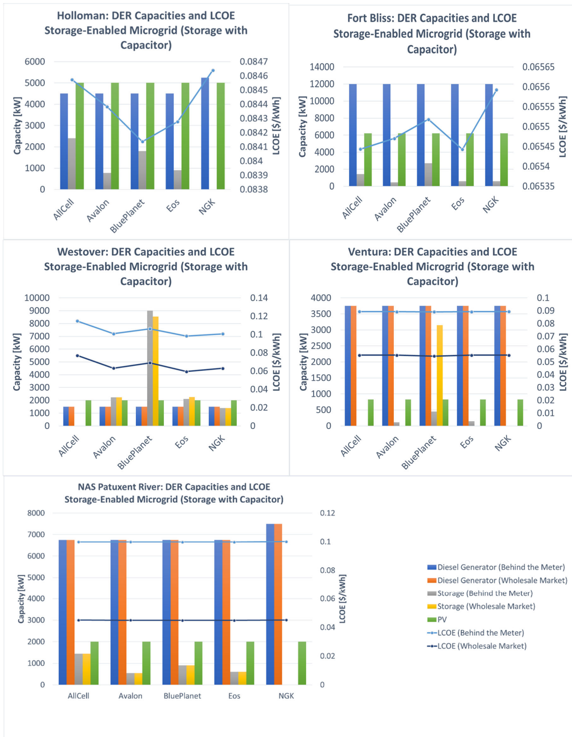
Figure ES-2b. Optimal Microgrid Portfolio and Levelized Cost of Electricity of Each Base Modeled for Each Battery Technology Paired with a Ultracapacitor/UPS System that Can Extend the Expected Life Including ITC and MACRS Incentives.
