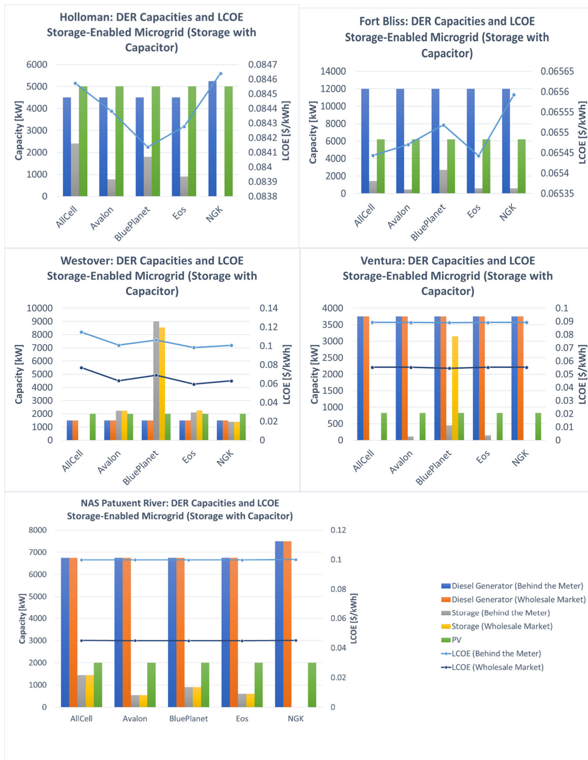
Figure 7. Optimal Microgrid Portfolio and Levelized Cost of Electricity of Each Base Modeled for Each Battery Technology Paired with a Ultracapacitor/UPS System that Can Extend the Expected Life Including ITC and MACRS Incentives.
