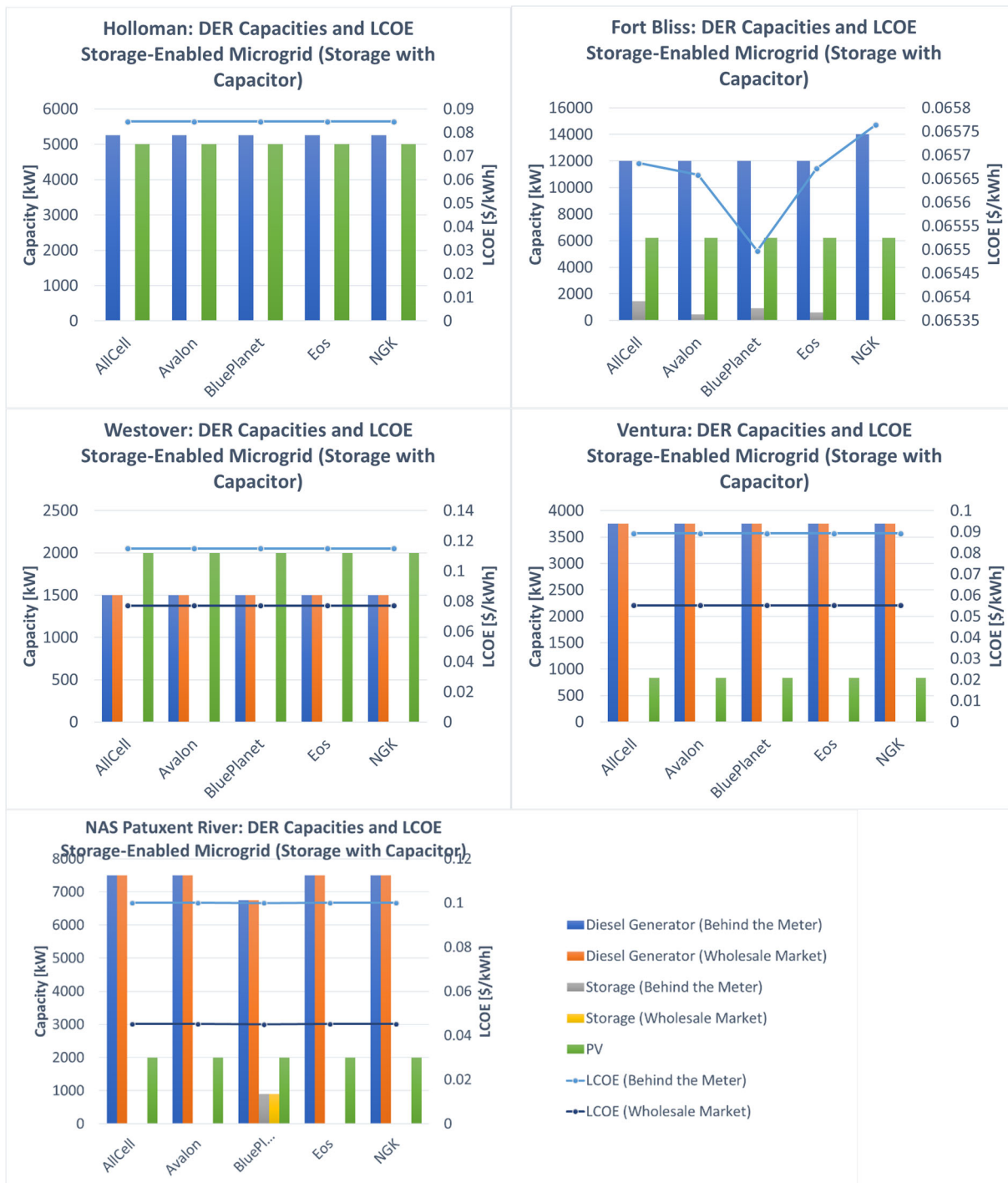
Figure 6. Optimal Microgrid Portfolio and Levelized Cost of Electricity of Each Base Modeled for Each Battery Technology Paired with a Ultracapacitor/UPS System that Can Extend the Expected Life with no ITC or MACRS Incentives.
