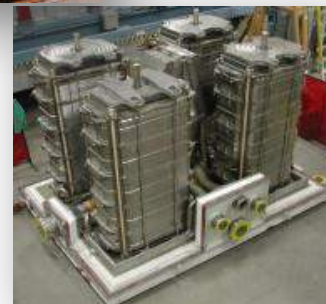
4 stacks are combined to build a 1.4 MW plant
